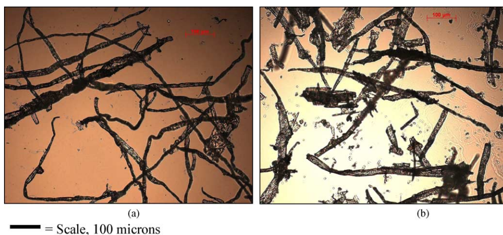
Fig. 2. Images from LF (a) and PPF fibres, obtained by optic microscopy. Scale = 100 \mu\text{g} .
